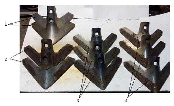
Fig. 3. Lancet paws after field work, reinforced with various electrodes: 1 - control; 2 - R5M6; 3 - T15K6; 4 - T-590
